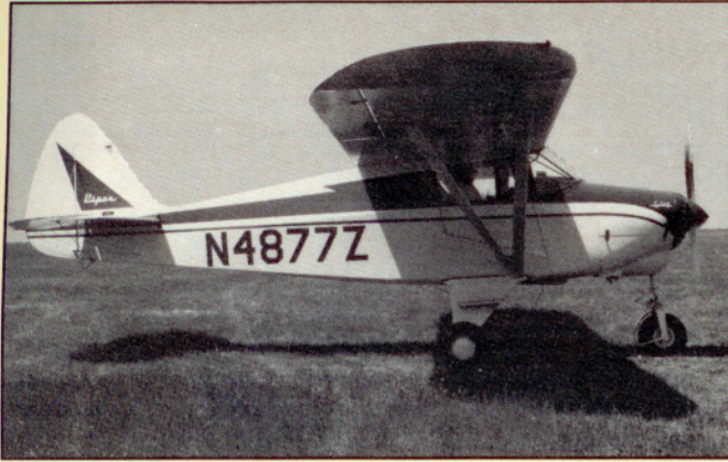
If you look closely at a Piper Colt of the early 1960s, you will discover that it is simply the PA-22 Tri-Pacer airframe with one door, no flaps and the 115-hp Lycoming O-235 engine of the PA-16.
