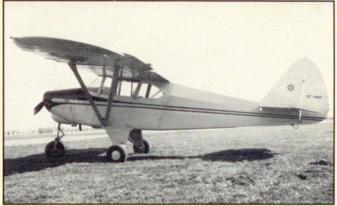
Originally offered only as an option, the Tri-Pacer became the principal production model of short-wing Pipers. This is an early model with the original designation, Pacer 125. Eventually, the designation became the Tri-Pacer 160.
