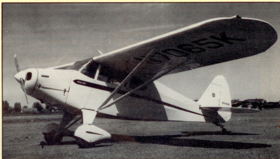
A copyright held on the name Clipper forced Piper to change its aircraft's name. Some improvements were made, and the result was the PA-20 Pacer. It had flaps, control wheels and a 125-hp Lycoming O-290D engine.
